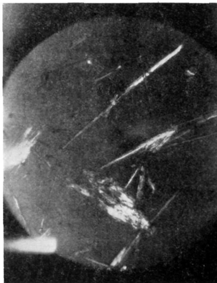
Illust. 5.— \text{Na}_2\text{Si}_2\text{O}_6 crystals originally from a melt but after long immersion in solution (partially crossed nicol prisms, 193\times ).
